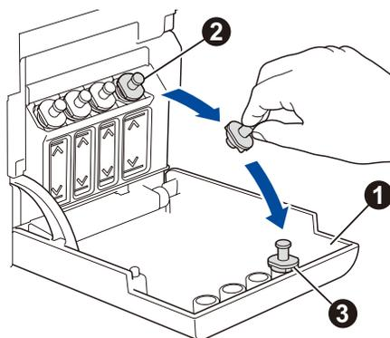
Open the ink tank cover 1, remove the cap 2, and place it on the back of the cover 3.
