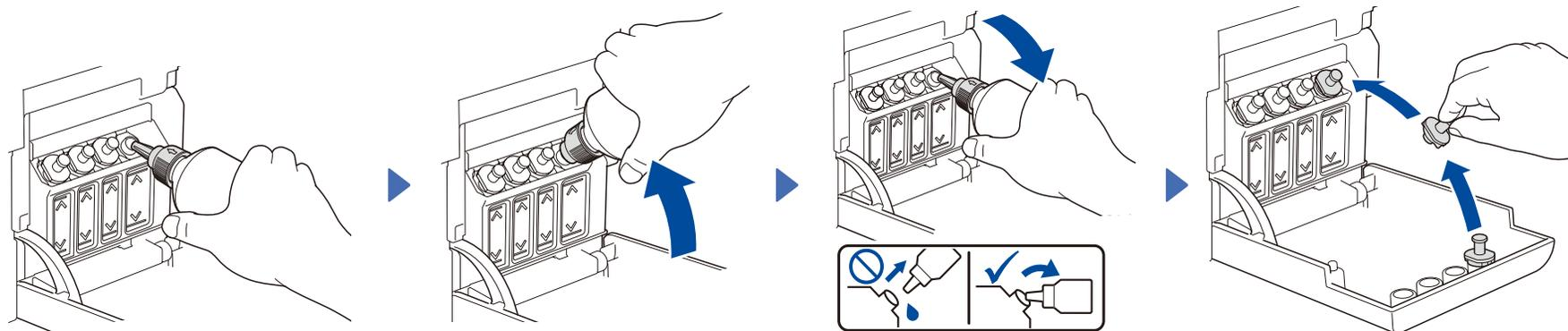
Remove the nozzle cap and insert the bottle nozzle firmly into the ink tank so that the ink does not spill.
