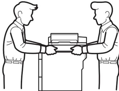
If you use a Lower Tray, DO NOT carry the product with the Lower Tray as you may be injured or cause damage to the product because it is not attached to the Lower Tray.
