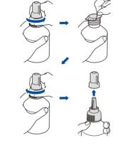
Remove the film and tighten the cap firmly.
