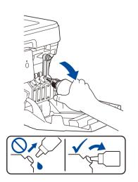
When finished, remove the bottle, pointing the nozzle upward so the ink does not spill.
