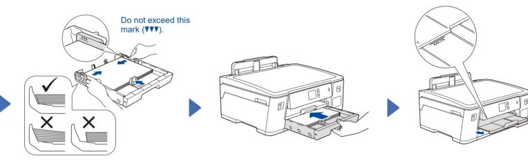
Pull the paper tray completely out of the machine as shown by the arrow.
