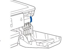
Push down on the cap of the ink tank to close it tightly. Repeat step 5 for the three other ink tanks.
