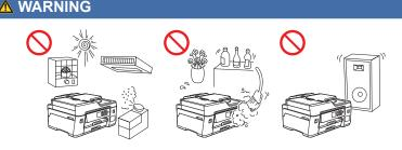
Choose a location where the temperature remains between 10°C and 35°C, the humidity is between 20% and 80%, and where there is no condensation.
