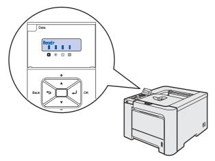
Press Go. The printer prints a test page. Check that the test page has printed correctly.
