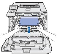
12 Make sure that the gray lock lever (1) is in the up position and put the drum unit in the printer. Push down the gray lock lever (1).
