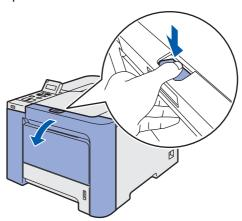
Hold the green handle of the drum unit. Lift the drum unit up and then pull it out until it stops.
