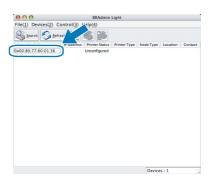
Choose **STATIC** for the **BOOT Method**. Enter the **IP Address**, **Subnet Mask** and **Gateway**, and then click **OK**.
