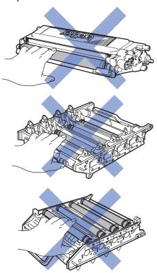
Attach the original orange protective cover to each of the toner cartridges. Place each of the toner cartridges into the plastic bag included in the carton.
