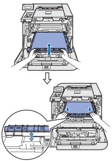
10 Insert the original orange packing material for locking the belt unit as shown in the illustration
