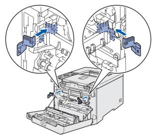
15 Two people should place the printer into the plastic bag and put the printer and the Styrofoam pieces into the carton. Match the front side of the printer to the "FRONT" mark (1) on the Styrofoam pieces. Put the Styrofoam piece for the toner cartridges (2) on top of the printer.
