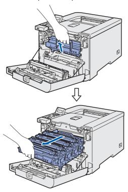
Release the gray lock lever (1) that is on the left side of the printer. Pull the drum unit completely out using the green handles on the drum unit.
