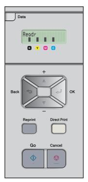
1 Press the + or – button until the LCD shows General Setup.
