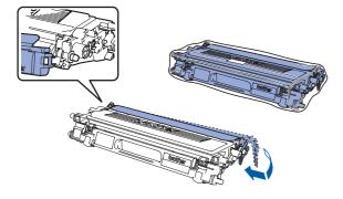
Hold the green parts of the belt unit with both hands and lift the belt unit up, then pull it out.
