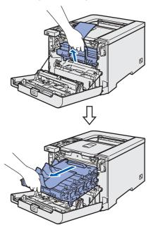
4 Remove the orange packing material as shown in the illustration below.
