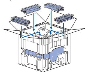
Put the two carton trays (1) (2) on the top and put the waste toner box in the tray placed towards the front side of the printer (1).
