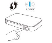
Press the WPS or AOSS<sup>™</sup> button on your wireless LAN access point/router.
