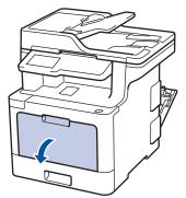
4. Pull out the MP tray support (1) and unfold the flap (2).
