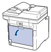
3. Pull the green levers at the left and right sides toward you to release the fuser cover.
