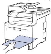
4. If paper is not jammed inside the machine, remove the paper from the paper tray, flip it over, and check underneath the paper tray.
