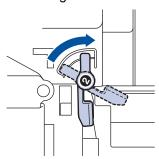
12. Using the green handle, push the drum unit back into the machine until it locks in place.
