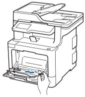
5. Load paper with the printing surface face up in the MP tray.
