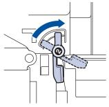
18. Using the green handle, push the drum unit back into the machine until it locks in place.
