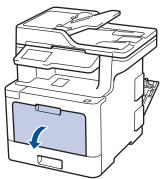
3. Pull out the MP tray support (1) and unfold the flap (2).
