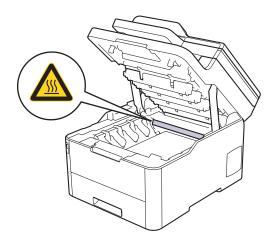
2. Remove the toner cartridge and drum unit assemblies.
