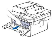
8. Turn the drum unit as shown in the illustration. Make sure that the drum unit gear is on the left side.
