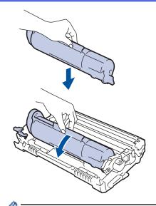
Make sure you put the toner cartridge in correctly or it may separate from the drum unit. If you put it in properly, the green lock lever will lift automatically.
