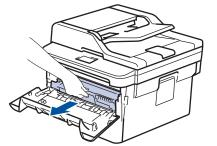
4. Push down the green lock lever, and then take the toner cartridge out of the drum unit as shown in the illustration.
