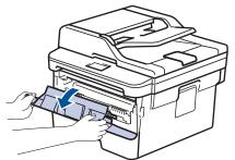
3. Remove the toner cartridge and drum unit assembly from the machine.
