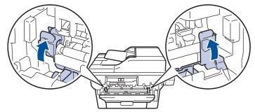
If you print on envelopes, pull down the green envelope levers to the envelope position again before closing the back cover.
