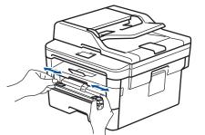
4. Using both hands, put one full sheet of paper in the manual feed slot until the front edge touches the paper feed roller. When you feel the machine pull it in, let go.
