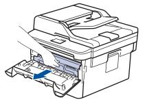
3. Clean the corona wire inside the drum unit by gently sliding the green tab from left to right and right to left several times.
