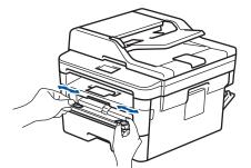
5. Using both hands, put one envelope in the manual feed slot until the front edge touches the paper feed roller. When you feel the machine pull it in, let go.
