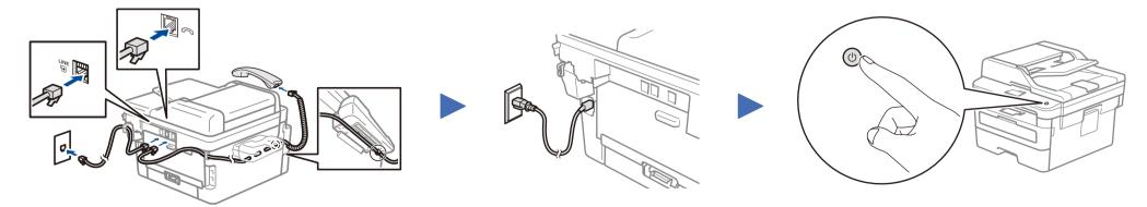
Connect telephone line and handset cord (Only for MFC-B7220DN/MFC-B7700D)
