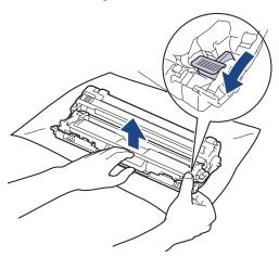
To avoid print quality problems, DO NOT touch any surface of the drum unit except the drum unit gear.
