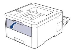
4. Use both hands to slide the manual feed slot paper guides to fit the width of the paper that you are using.
