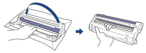
9. Loosen your grip so the frame drops forward, and then use your right hand to locate the drum unit gear inside the right side of the frame.
