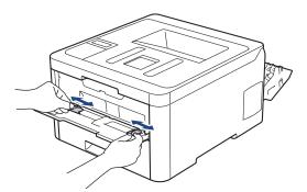
5. Using both hands, put one envelope in the manual feed slot until the front edge touches the paper feed roller. When you feel the machine pull it in, let go.
