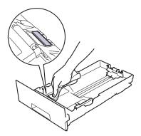
5. Wipe the two pick-up rollers inside the machine to remove dust.
