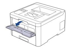
3. Use both hands to slide the manual feed slot paper guides to fit the width of the paper you are using.
