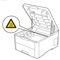
6. The colour of printed dots on the Drum Dot Check Sheet is the colour of the drum you should clean. Remove the toner cartridge and drum unit assembly that matches the colour causing the problem.
